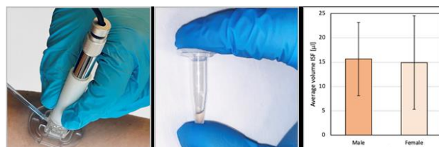
Figure 1. Sampling tool (left), 32 \mu\text{l} sampled dISF (middle), and comparison between sampled volumes (right).
